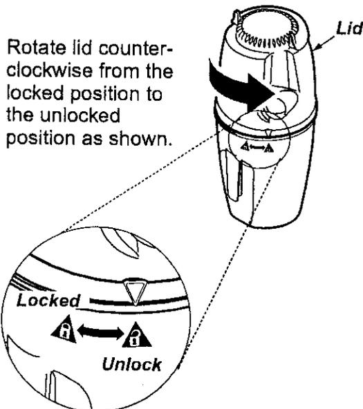
Rotate lid counter-clockwise from the locked position to the unlocked position as shown.
